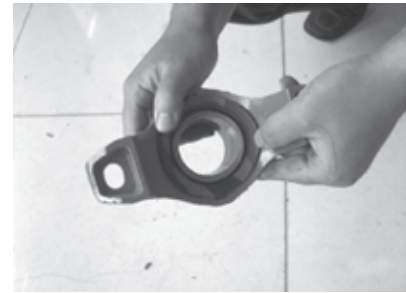
3. Put gasket seal in the Mechanical Tee.
